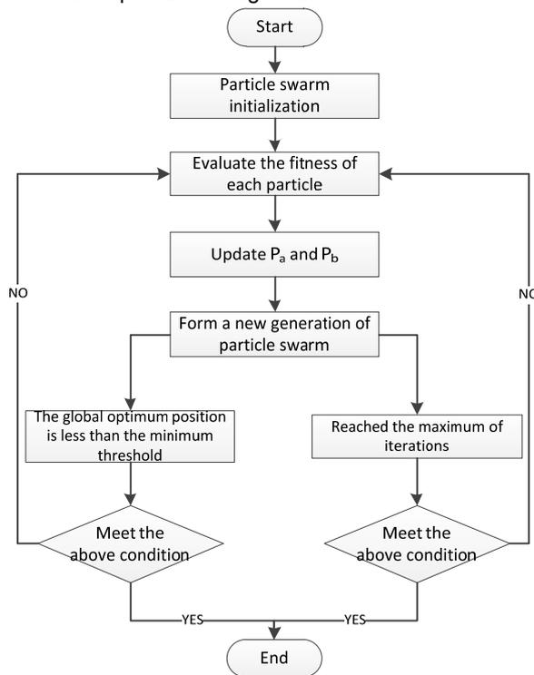
Figure 1: Flow chart of particle swarm optimization algorithm
