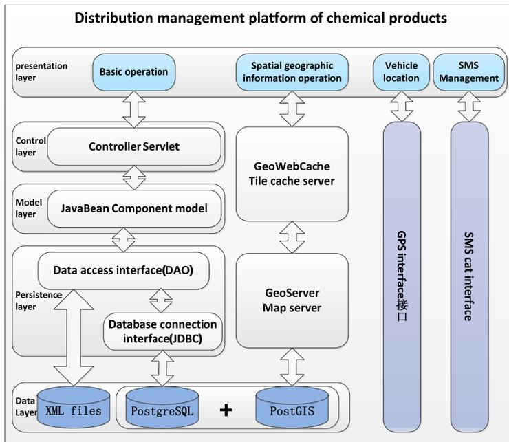
Figure 2: System architecture of distribution management platform
