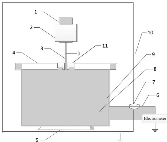
Figure 2: Spinning round disk system. 1: encoder; 2: DC motor; 3: rotating mandrel; 4: cover; 5: insulator; 6: coaxial cable; 7: insulator; 8: disk; 9: oil; 10: Faraday cage; 11: insulator.
