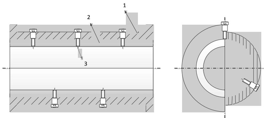
Figure 4 Structure of electrostatic neutralization device for oil pipeline. 1: steel pipe; 2: insulator; 3: discharge pin.
