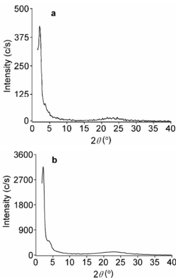
Figure 1: XRD spectra of mesoporous silica and silane mesoporous silica
