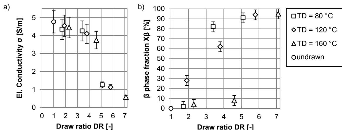
Figure 5: a) Electrical properties of the fibers drawn at different temperatures as a function of draw ratio, b) fraction of the piezoelectric crystalline phase ( $\beta$  phase) for fibers drawn at different temperatures as a function of draw ratio
