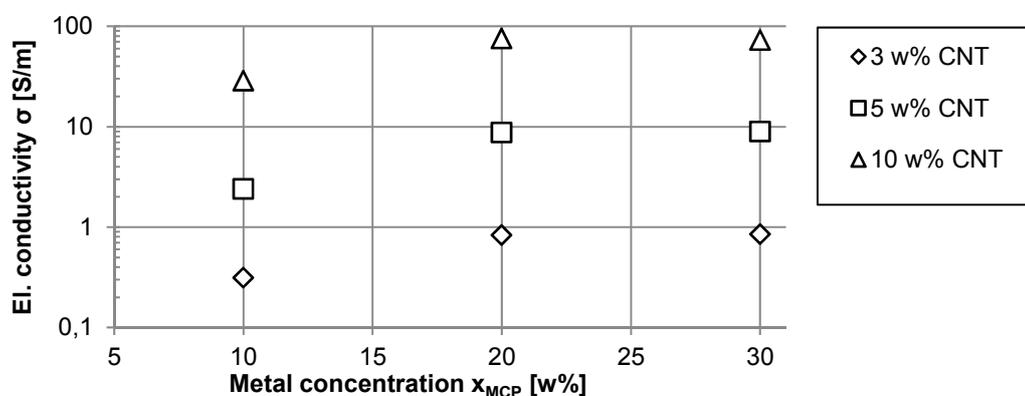
Figure 2: Electrical properties of the compounds (PP/CNT/MCP220)
