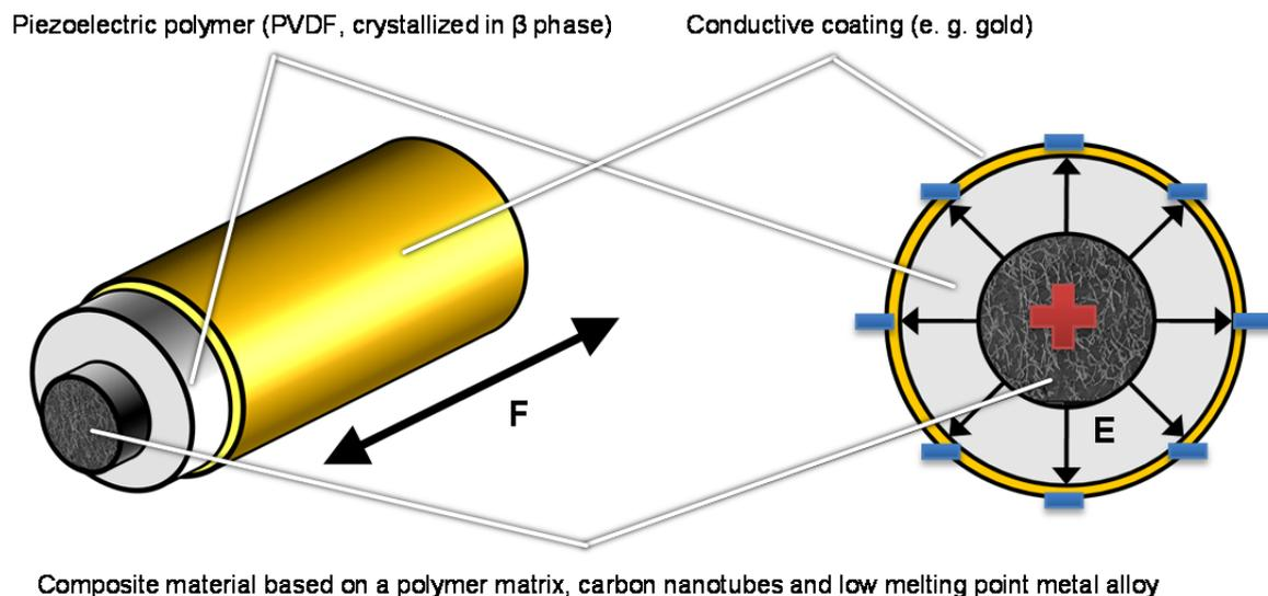
Figure 1: Concept for piezoelectric sensor fibers
