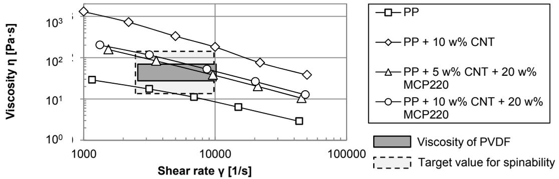
Figure 3: Rheological properties of the compounds (PP/CNT/MCP220)
