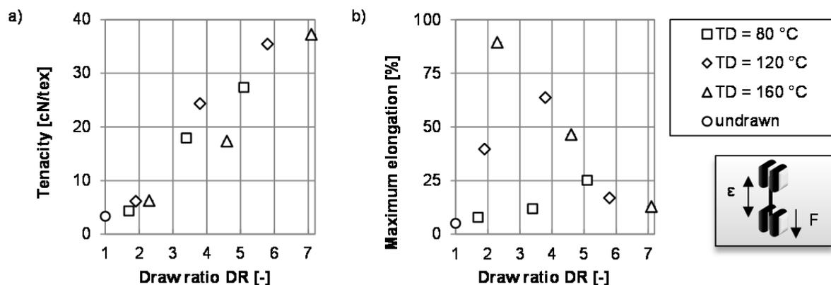
Figure 4: Mechanical properties of the fibers drawn at different temperatures, a) Tenacity as a function of draw ratio, b) Maximum elongation as a function of draw ratio#
