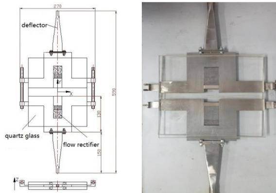
Figure 1: Schematic diagram of the experimental apparatus
