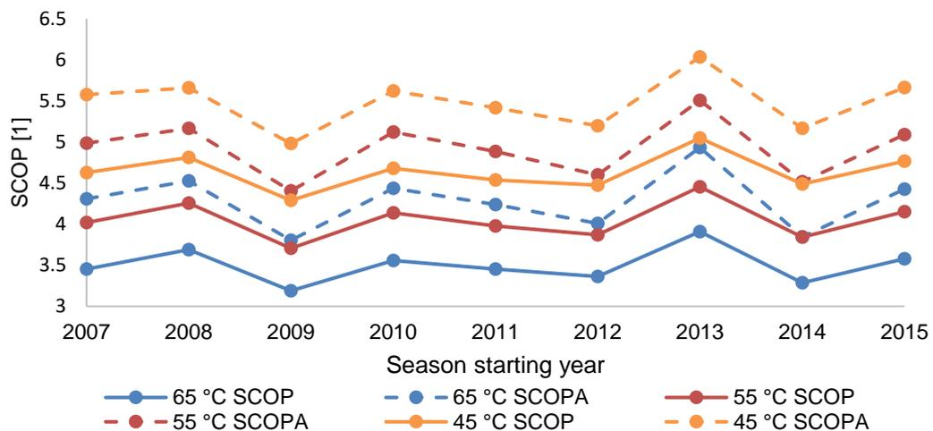
Figure 5: Identified SCOP and SCOP<sub>A</sub> in heating seasons 2007-2016
