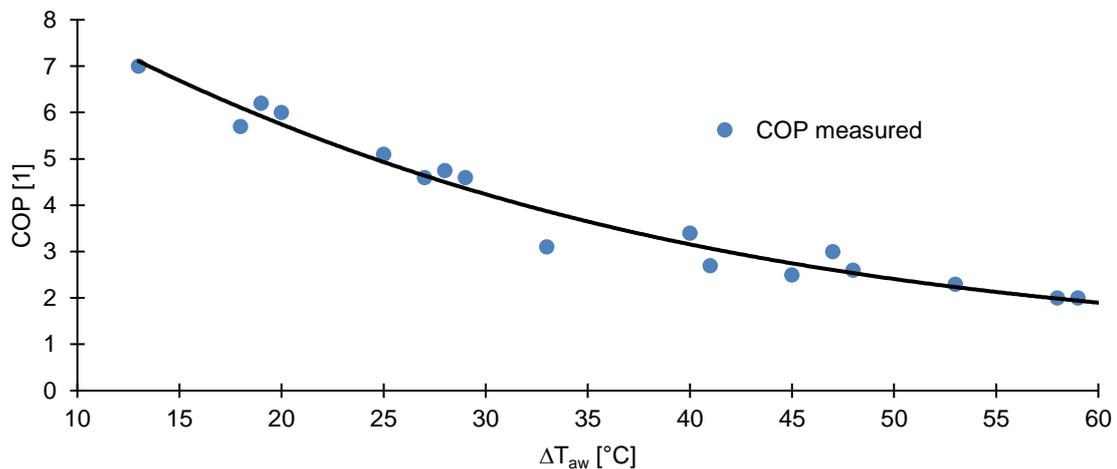
Figure 3: Dependency of COP on the temperature difference  $T_{aw}$
