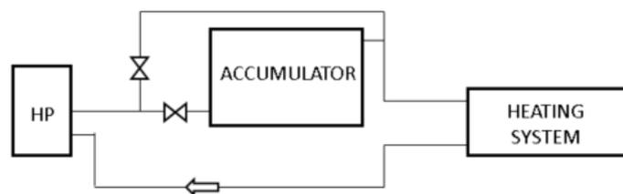
Figure 4: System with a flow volume accumulator
