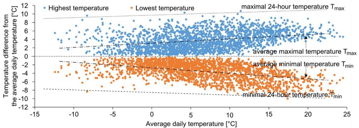
Figure 2: Relation of maximal/minimal air temperature during 24-h interval and average air temperature, heating seasons 2007-2016
