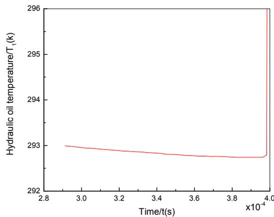
Figure 2: The change of hydraulic oil temperature during bubble compression
