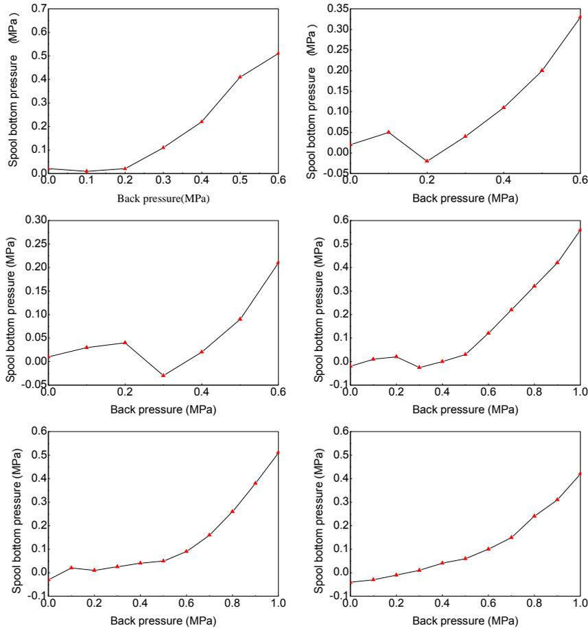
Figure 4: The change of the pressure at the bottom of valve core with back-pressure
