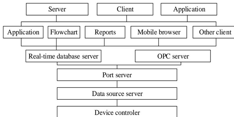
Figure 1: Production application framework for production monitoring system
