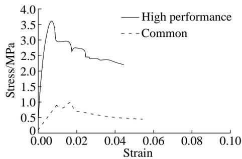
Figure 6: Uniaxial compression mechanical property of foam concrete
