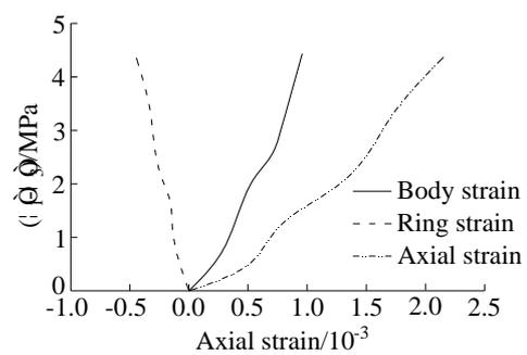
Figure 9: Triaxial mechanical properties of foam concrete under dynamic conditions
