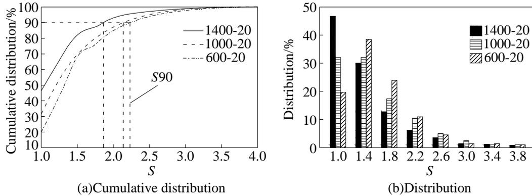
Figure 4: Shape factor for chemical foaming foam concrete at Three Density grades
