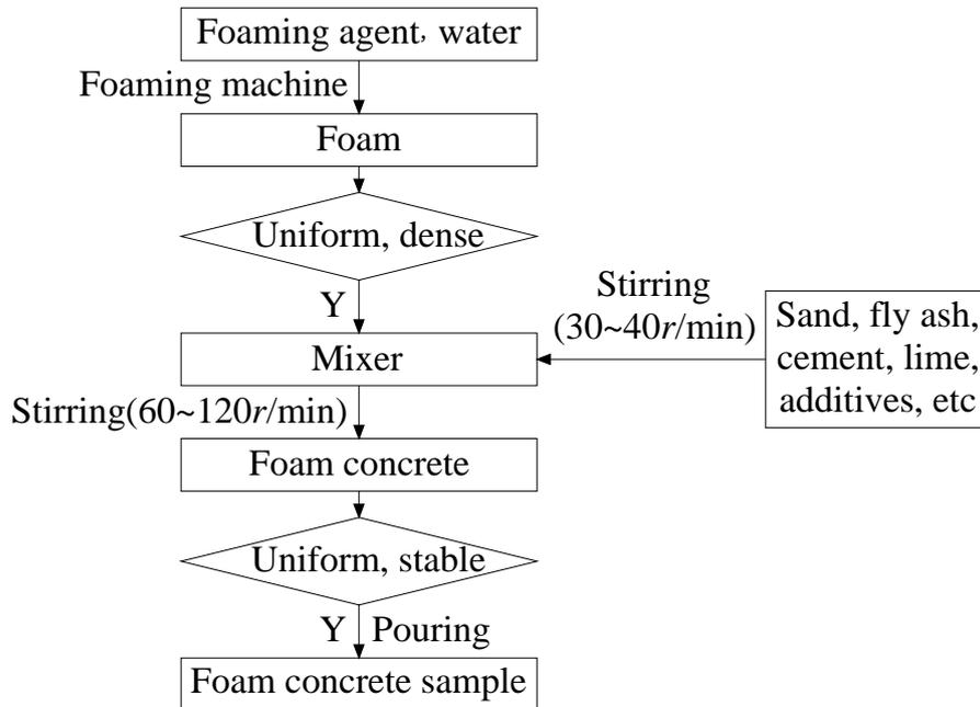
Figure 1: Chemical foaming foam concrete preparation process
