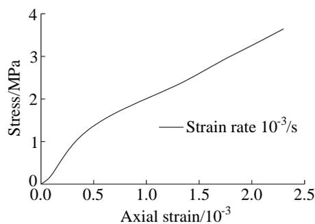
Figure 8: Uniaxial mechanical properties of foam concrete under dynamic conditions
