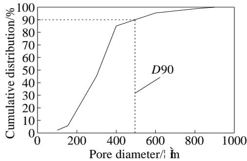
Figure 2: The cumulative pore size distribution of chemical foaming foam concrete
