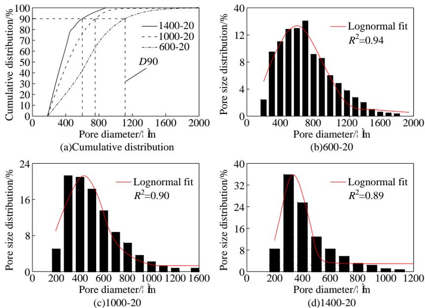
Figure 3: Pore size distribution of chemical foamed Foam concrete with three density grades
