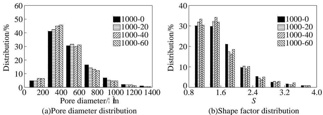
Figure 5: Effect of fly ash content on the pore size of concrete
