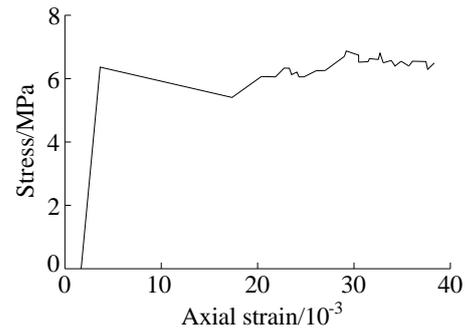
Figure 7: Axial mechanical properties of foamed concrete under hydrostatic pressure
