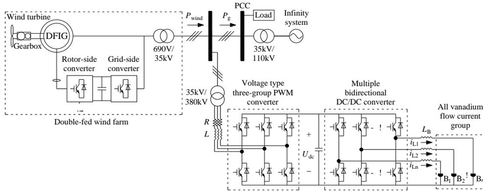
Figure 3: Architecture of wind power plant based on VRB energy storage technology
