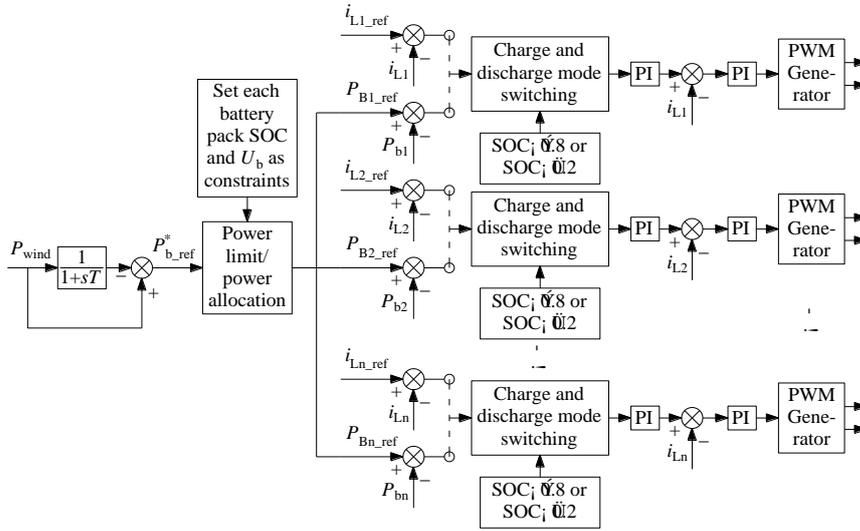
Figure 5: Control architecture of multiple AC and DC voltage converter
