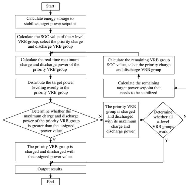
Figure 6: Optimal allocation scheme of multi-VRB energy storage
