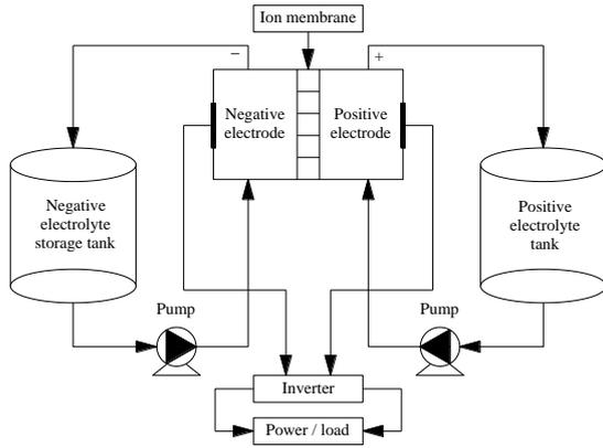
Figure 1: Working principle of VRB system
