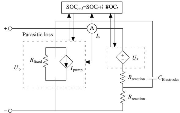
Figure 2: Equivalent circuit of VRB
