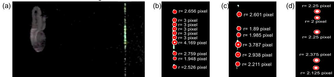
Figure 3: (a) An image of the spray coating process; image analysis results of the droplet at spray distance; (b)  $L = 10$  cm; (c)  $L = 20$  cm (c); (d)  $L = 30$  cm
