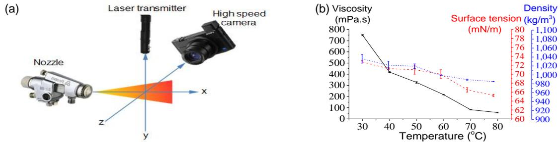
Figure 1: Diagram of the device to record the images (a) and change of polymer solution parameters according to temperature (b)
