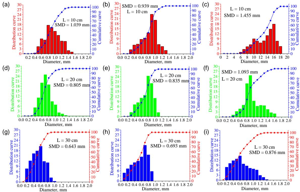
Figure 4: Distribution of droplet size corresponding to spray distances at experimental conditions as Table 4 with experiment No. 1 (a, d, g), No. 2 (b, e, h) and No. 3 (c, f, i)
