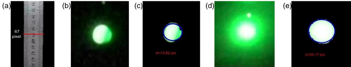
Figure 2: (a) An image of a ruler; (b) an image of a droplet; (c) results on image analysis of droplet; (d) an image of the laser light scattering droplet and; (e) result on image analysis of laser light scattering droplet.
