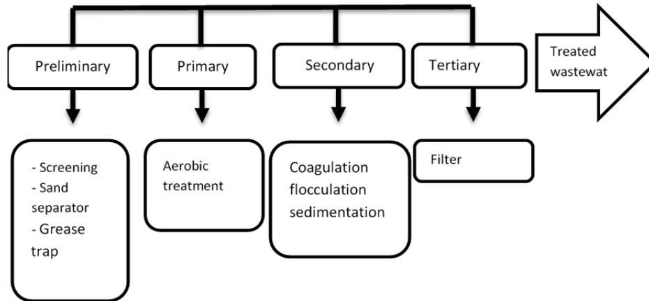
Figure 2: Process 2 Water treatment with aerobic reactor included.
